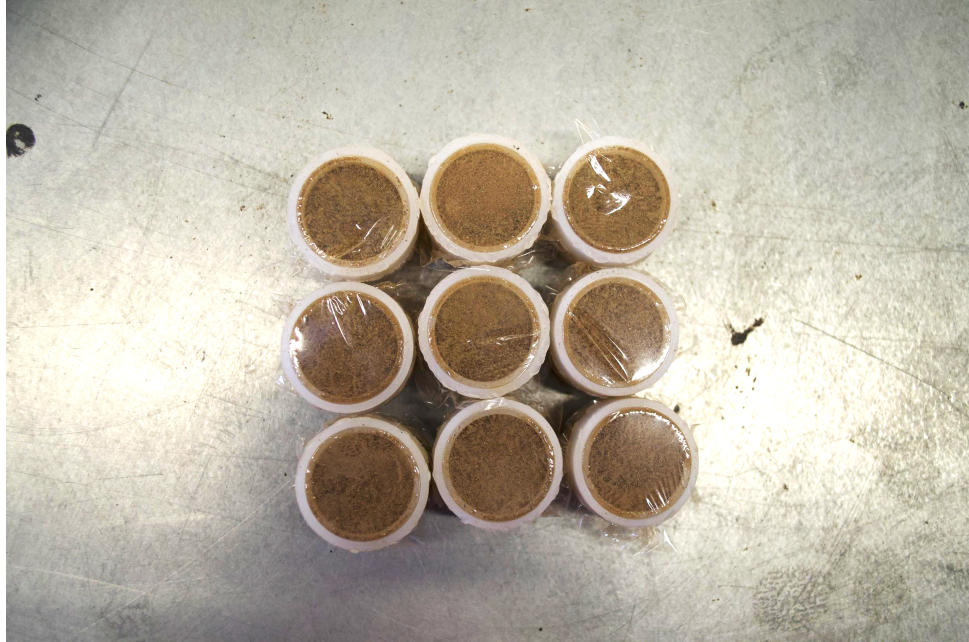
Figure 4-3. Soil Samples Prepared for XRF Analysis Divided into subsamples.
